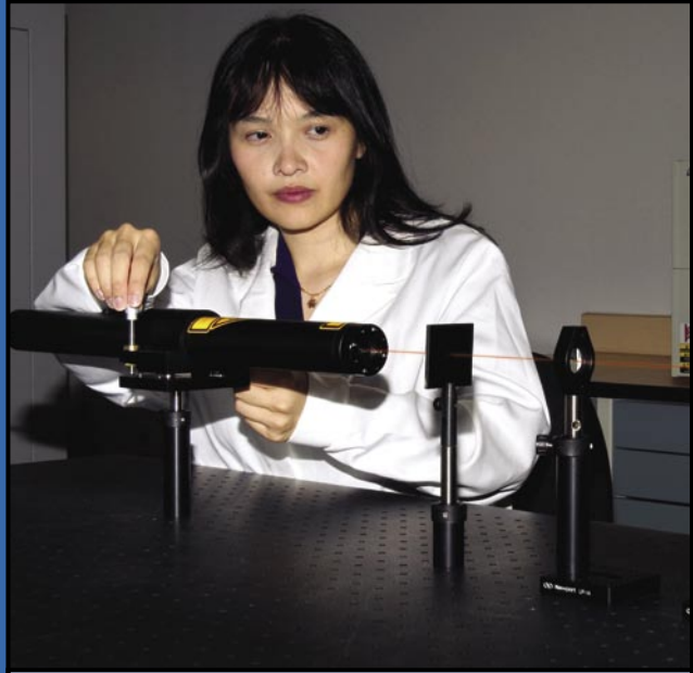
Dr. Ressejac is working with the characterization setup of closed loop two-DOF micromirrors. PHOTO: Canadian Space Agency
