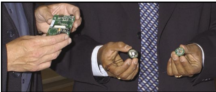
An electronic circuit called a "mote" (the circular object in the middle) connects to biosensors (mounted on the circular object on the right) to continuously monitor a patient's vital signs in real time. The sensed information is transmitted over radio to a base-station (the object on the left) that connects to a doctor's PC.
