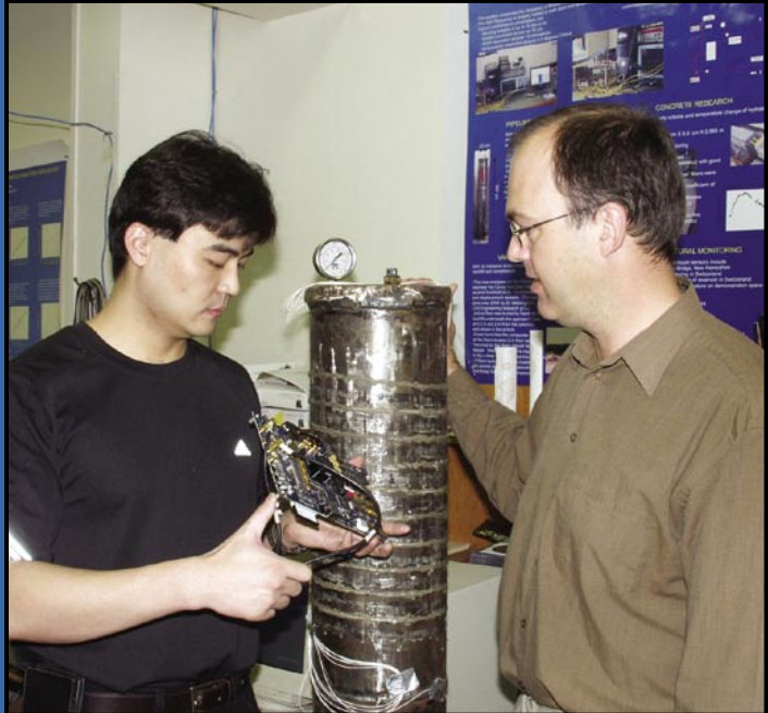
Dr. Bruce Colpitts, Professor, Electrical and Computer Engineering, UNB (right) is working with Ethan Zheng, graduate student (left) on an experimental technology that can detect rapid strain change or vibration in bridges, buildings or other structures.
